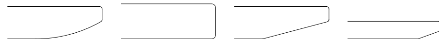
Solid wood edging, rounded on the bottom, straight plastic edging, chamfered wood edging or chamfered HPL solid-core edging
